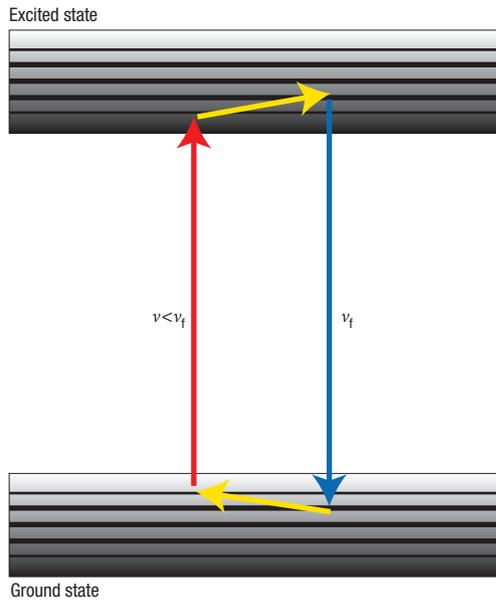
**Figure 1** An energy diagram showing one way anti-Stokes fluorescence could occur. An atom with two broad levels is embedded in an otherwise transparent solid. The light source of frequency  $h\nu$  (red arrow) excites atoms near the top of the ground-state level to the bottom of the excited state. Radiative decays, following interaction between the electrons and phonons (yellow arrows), emit photons with average energy  $h\nu_f > h\nu$  (blue arrow).
