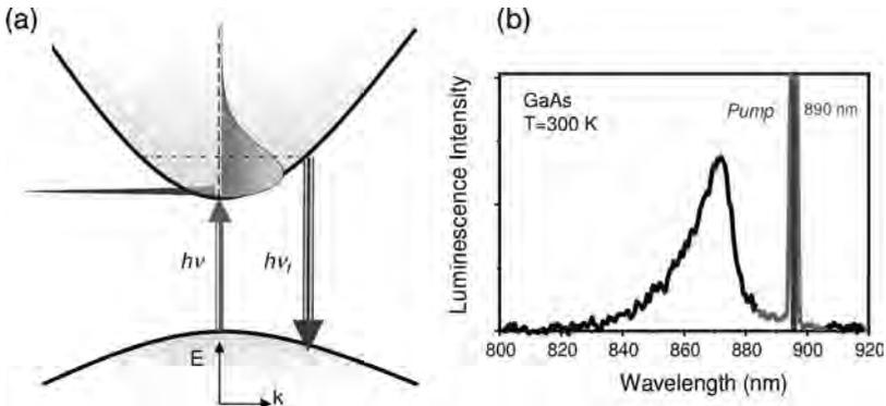
**Figure 1.8** (a) Cooling cycle in the laser refrigeration of a semiconductor in which the absorption of laser photons with energy  $h\nu$  creates a cold distribution of electron–hole carriers (only the electron distribution is
