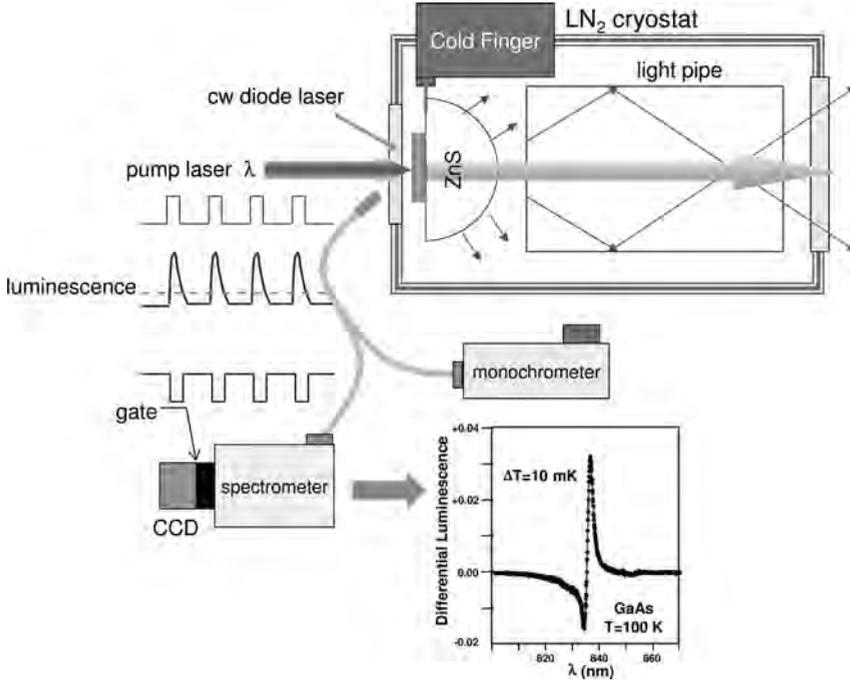
**Figure 1.14** Experimental setup for measuring the external quantum efficiency (EQE or  $\eta_{ext}$ ) at various lattice temperatures in GaAs/GaInP double heterostructures. A tunable cw laser (Ti:sapphire, 4.5 W) excites a constant density of electron-hole pairs as the pump is tuned near the band edge. This is done by keeping the luminescence intensity (within a certain spec-
