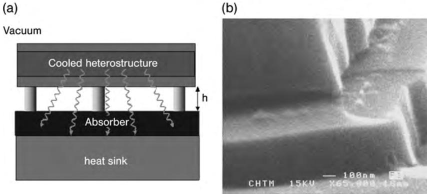
**Figure 1.17** (a) A vacuum “nanogap” structure where the heterostructure is situated (e.g. supported by posts) at a subwavelength distance from an absorber. Luminescence photons will escape into the absorber via frustrated total internal reflection (photon tunneling),
