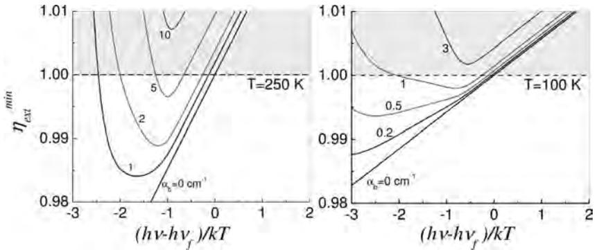
**Figure 1.10** The minimum EQE required to achieve laser cooling versus the normalized excitation photon energy for GaAs at  $T = 250$  and  $100$  K, obtained from the inequality of (1.29). The absorption data  $\alpha(\nu)$  were obtained by using the KMS relations on the
