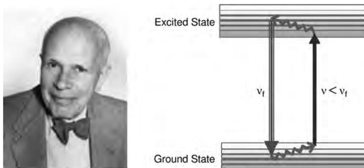
**Figure 1.1** In 1929, Peter Pringsheim suggested that solids could cool through anti-Stokes fluorescence, in which a substance absorbs a photon and then emits one of greater energy. The energy diagram on the *right* shows one way in which this could occur. An atom with
