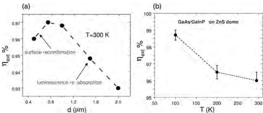
**Figure 1.15** External quantum efficiency (EQE) measured with (a) a bonded sample with various GaAs thicknesses, the GaInP layer thickness fixed at 0.5  $\mu\text{m}$ , and  $T = 300 \text{ K}$ , and (b) measured EQE vs. lattice temperature for a GaAs thickness of 1  $\mu\text{m}$ .
