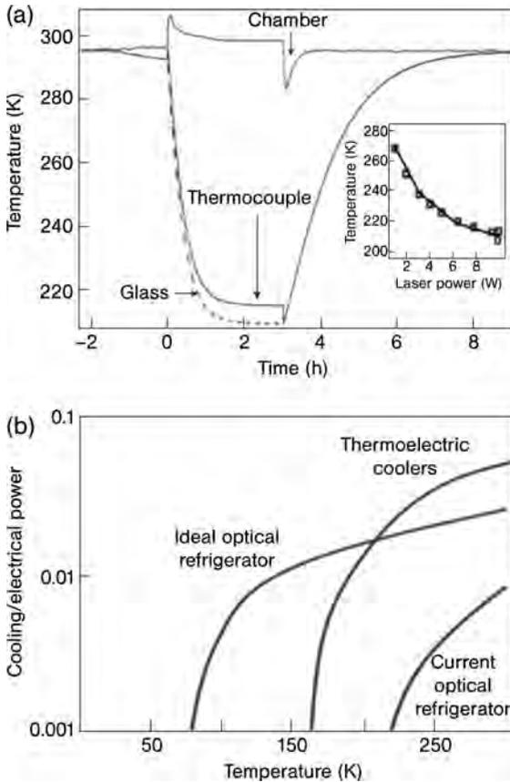
**Figure 1.5** Panel (a) shows record cooling to 208 K with ZBLANP:Yb<sup>3+</sup>. The temperatures are measured with thermocouples on the sample and chamber; the internal temperature of the glass is inferred [22]. Panel (b) compares the cooling efficiencies of available thermoelectric coolers (TECs)
