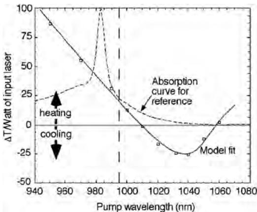
**Figure 1.4** The temperature change (normalized to the incident power) in ytterbium-doped ZBLANP glass as a function of pump wavelength. When the pump wavelength is considerably longer than the mean wavelength of the fluorescence  $\lambda_F$  (vertical dashed line),
