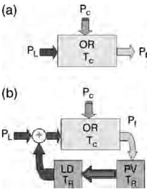
**Figure 1.18** Diagrams of (a) an open loop optical refrigerator (OR) and (b) a closed loop system in which the luminescence (photon waste) recycling is performed using photovoltaic (PV) elements followed by a laser diode (LD), both at a temperature  $T_R$ .
