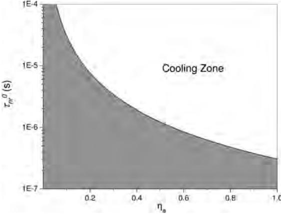
**Figure 1.9** The break-even nonradiative lifetime as a function of the luminescence extraction efficiency in bulk GaAs, calculated using typical values of radiative and Auger recombination at room temperature.
