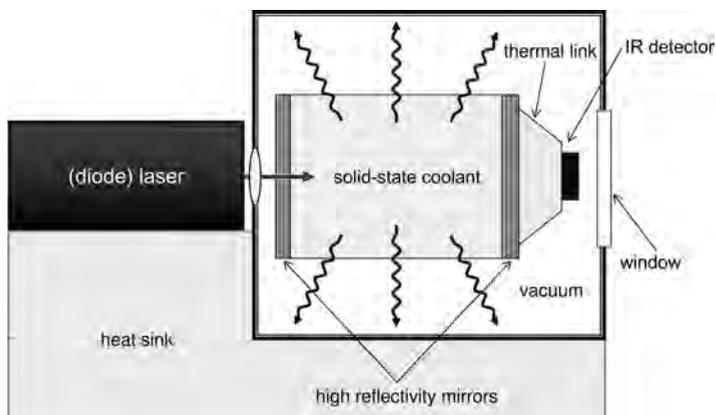
**Figure 1.2** Schematic of an optical refrigeration system. Pump light is efficiently generated by a semiconductor diode laser. The laser light enters the cooler through a pinhole in one mirror and is trapped by the mirrors until it is absorbed. Isotropic fluorescence
