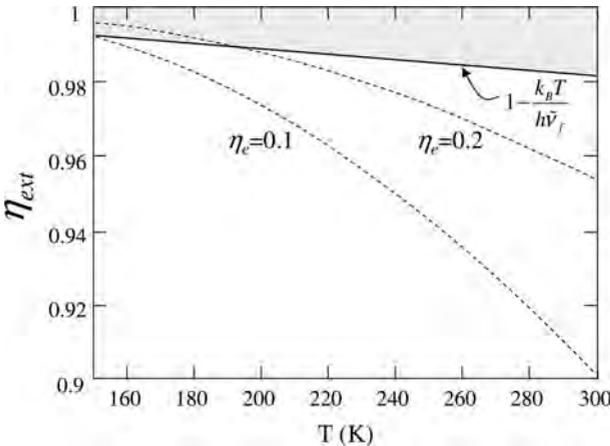
**Figure 1.11** The required external quantum efficiency (EQE) as a function of temperature for GaAs under typical parameters.
