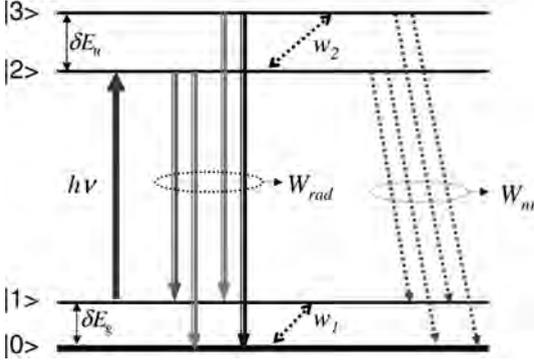
**Figure 1.3** The four-level energy model for optical refrigeration consisting of two pairs of closely spaced levels:  $|0\rangle$  and  $|1\rangle$  in the ground state and  $|2\rangle$  and  $|3\rangle$  in the excited-state manifolds.
