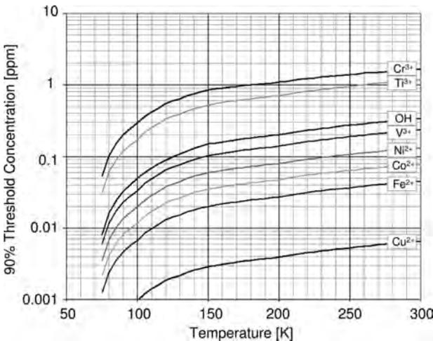
**Figure 1.6** Calculated impurity threshold concentrations. If the impurity level of an ion is above the level shown here, the cooling efficiency of the ZBLAN:1%Yb<sup>3+</sup> will be less than 90% of its ideal value and rapid heat conversion can occur. See the detailed study by Hehlen *et al.* [39].
