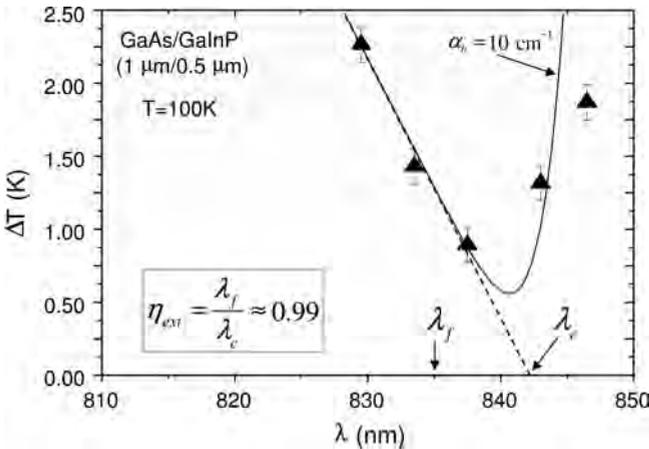
**Figure 1.16** Fractional heating of a  $1 \mu\text{m}$  thick GaAs sample as a function of excitation wavelength for a fixed (optimum) electron–hole density at a starting temperature of 100 K. The extrapolation of short-wavelength data determines the zero-crossing wavelength, from which a record EQE of  $\sim 99\%$  is measured. Excitation at longer wavelengths causes heating due to background parasitic absorption [6, 68].
