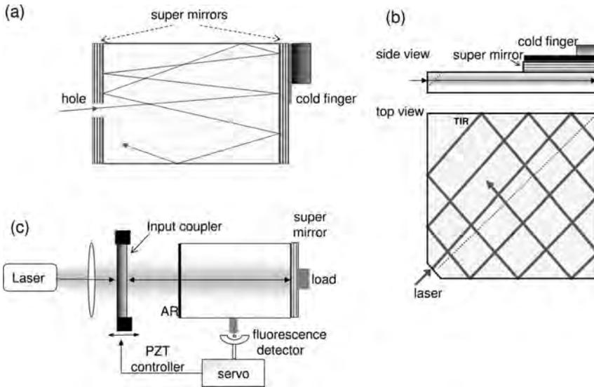
**Figure 1.7** Methods to enhance pump absorption. (a) Non-resonant cavity formed by dielectric mirrors deposited on the sample. The pump laser enters through a small hole in one of the mirrors. (b) Nonresonant cavity based on total internal reflection, in which the laser enters through a bevel. (c) Cavity-enhanced absorption, where light couples through a matched dielectric mirror. This required active stabilization.
