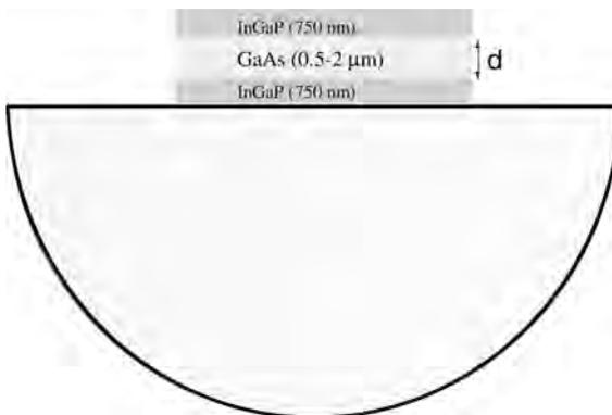
**Figure 1.13** The GaAs/GaInP double heterostructure is bonded to a nearly index-matched dome (ZnS or ZnSe) to enhance its luminescence extraction.
