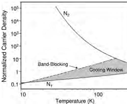
**Figure 1.12** The upper carrier density  $N_2$ , given by (1.26), is seen to be unattainable in GaAs due to band blocking as the temperature is lowered below 200 K. The *middle (dashed) line* represents the calculated density at which the band-tail absorption at  $h\nu = h\nu_f - k_B T$  completely saturates (i.e.  $\alpha(N) = 0$ , (1.10)). This is a worst case scenario for which the nonradiative recombination rate is assumed to be constant with temperature.
